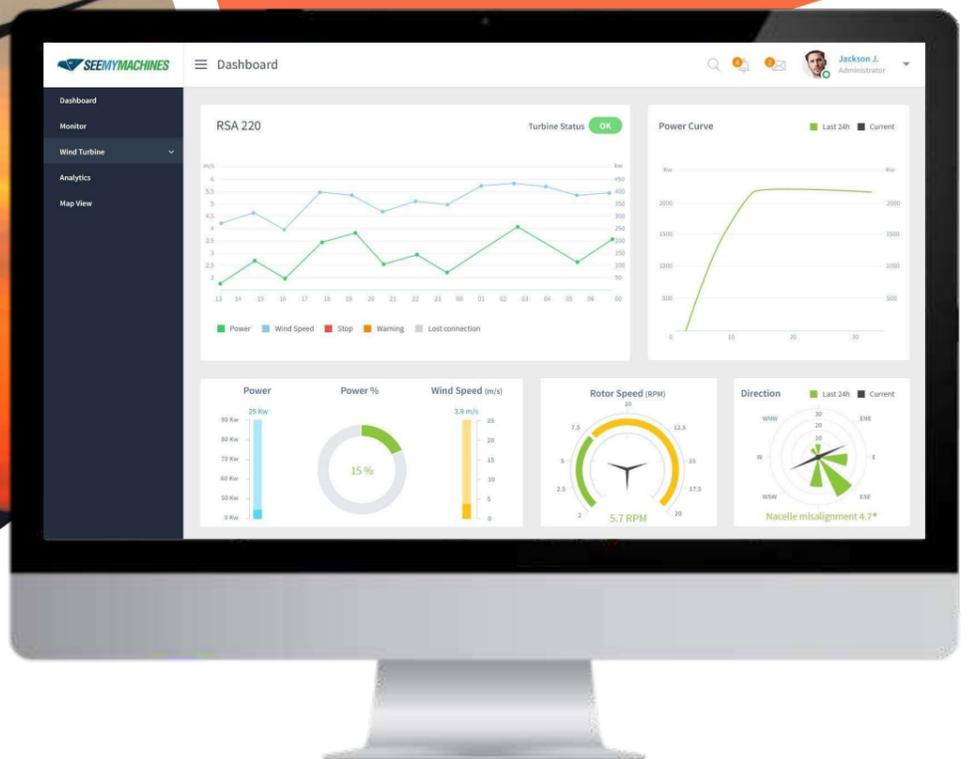
A cloud-based IoT solution with advanced analytical capabilities for condition monitoring and performance tracking of equipment at wind farms.
